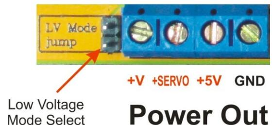
The 5V regulator will get much hotter in this mode so the 5V current should be limited to 800mA unless a heatsink and fan are added directly to the LM1084 regulator IC.
