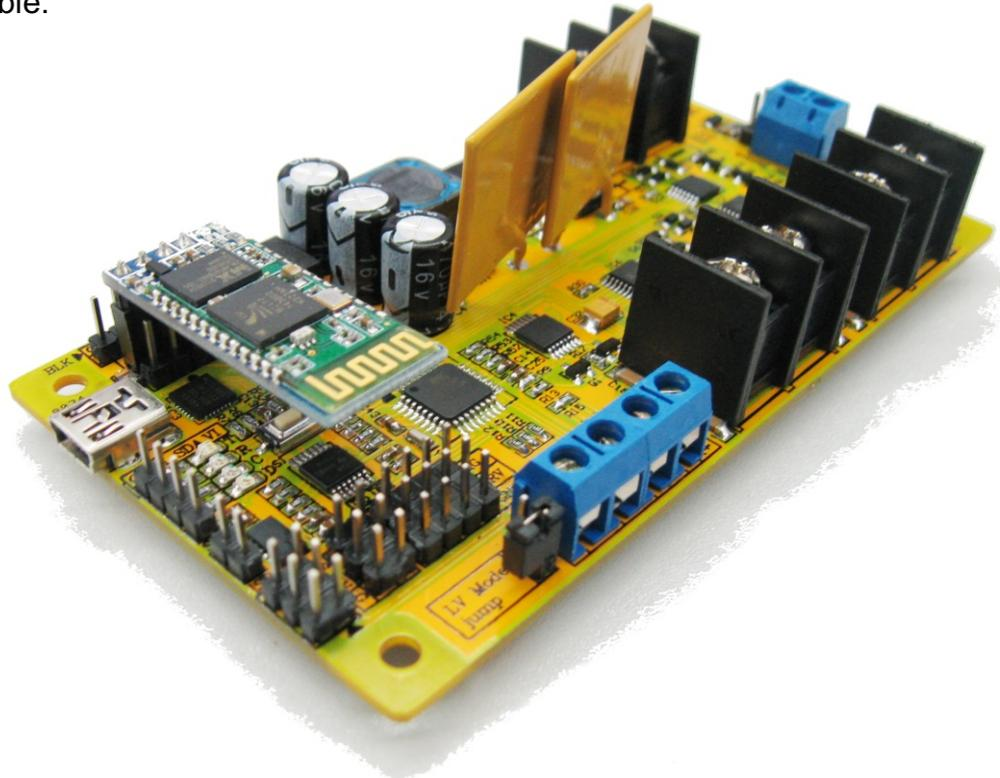
If the bluetooth module is detected the sample code will automatically set the baud rate to 9600, the name to “T'REX” and the pin number to “1234”.
