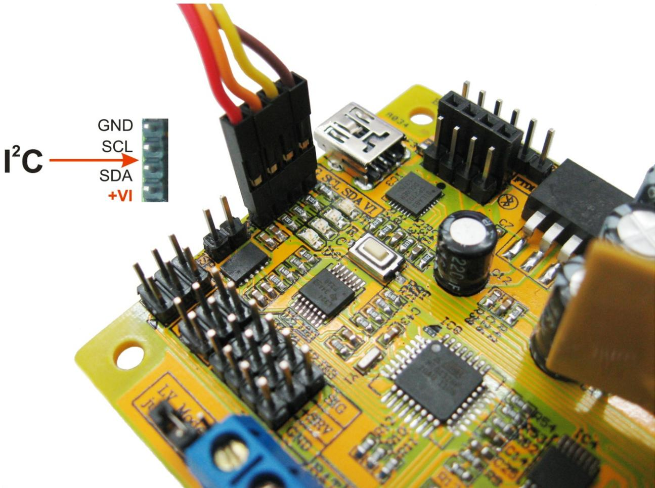
Connect the +V, SCL, SDA and Gnd of the external logic to the +VI, SCL, SDA and GND pins of the T'REX I<sup>2</sup>C interface. The T'REX will automatically translate the voltage. The interface includes 10K pullup resistors although external pullup resistors can be added if required.
