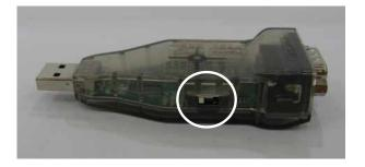
Set the function select switch to TTL mode.
