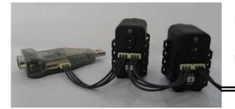
By using the 3P cable, Dynamixel can be daisy chained.
