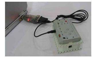
CM-5 uses a serial port to communicate. By using USB2Dynamixel, users can communicate with CM-5 via USB port. For more details, refer to the Bioloid manual.
