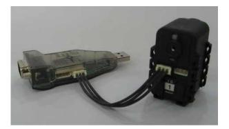
Connect 3P cable to the 3P connector of USB2Dynamixel and Dynamixel connector (either one can be connected).
