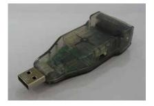
Use to directly operate Dynamixel from PC. Or when converting a USB port to a serial port.
