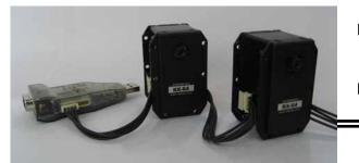
By using the 4P cable, Dynamixel can be daisy chained.
