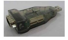
USB2Dynamixel is a device that can directly control Dynamixel from PC. 3P connector and 4P connector are built-in, allowing USB2Dynamixel to connect to various Dynamixels and it is used by connecting to a USB port.
