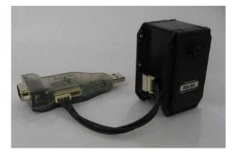
Connect 4P cable to the 4P connector of USB2Dynamixel and Dynamixel connector (either one can be connected).
