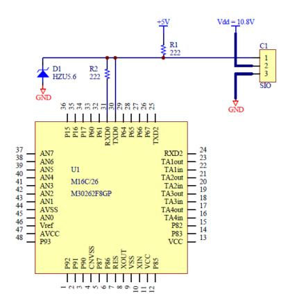
To enable half-duplex operation, TXD (transmission) and RXD (receiving) lines are tied together on the microcontroller side of the circuit and are connected to the signal pin (number 1) on the SIO connector. The system uses a negative logic circuit, so to keep the signal at 5V, a  $2.2k\Omega$  pull-up resister (R1) is used. RXD is an input signal - and so to prevent damaging the CPU from electrical noise or electrostatic discharges, a resister (R2) is placed in series.
