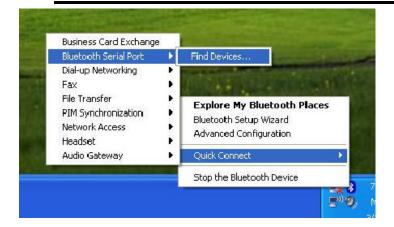
Click on "Quick Connect" to "Bluetooth Serial Port" to "Find Devices". After a minute or so of searching, you should see this:
