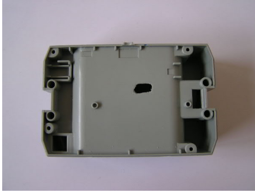
Hole Drilled in Plastic Battery Box of CM-5
