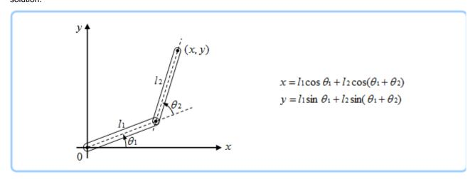
On the other hand, inverse kinematics may be used to determine the angle or movement of the joint from the location or movement of the end point. For example, suppose again that there is a manipulator with two joints in the same plane coordinates. If the end point (x,y) has been determined, there are 2 possible values for each joint as seen below.
