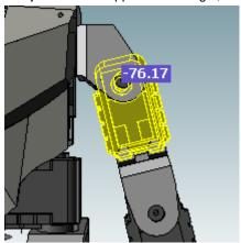
If you move the mouse to left and right while pressing the left botton of the mouse, the value increases or decreases. In case of 1024-based control, the unit of the value is approximately 0.29(300 / 1024), and in case of 4096-base, it is approximately 0.06(250.92 / 4096).
