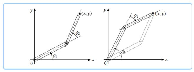
When using inverse kinematics, the coordinate (x,y) of the end point may be located at an unreachable distance from the origin or no solution may be obtained due to limitations on joint angles. If more joints are used, there may be infinitely many solutions.
