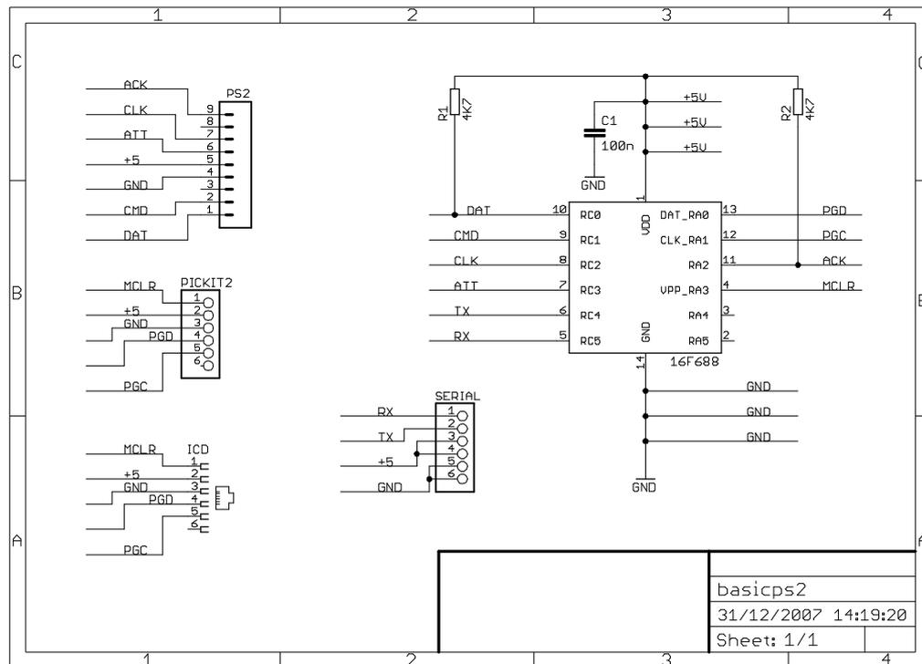
**5) Building the converter** I choose to build the converter with a DIP PIC 16F688 on a scrap of prototype board. The board was only slightly larger than the DIP chip to include the capacitor and resistors, no IC socket was used. The wires for the cables went direct to the IC pins. I used a 3 pin servo connector to give access to the programming pins in the PIC. Then put it in heat shrink sleeving.
