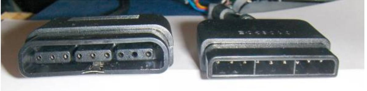
The photo above shows the connector on the receiver on the right, and the socket it plugs into on the left. There are nine pins to the connector, but only seven are used.
